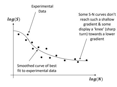
Fatigue strength is a hypothetical value of stress range at failure for exactly N cycles as obtained from an S-N curve.
