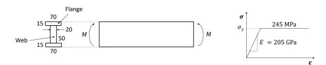
Yielding will occur through whole of flange and 5 mm into each end of the web, therefore:
